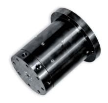
The shaft, which is manufactured in the shape of a flange, is divided into single and double types. In case of the double type, two rotaries are turned individually or concurrently as necessary on the same shaft.
