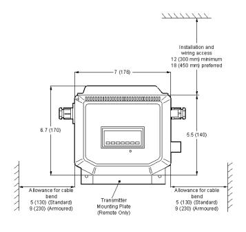
**Note:** For Integral mounting, the Electronic Display Unit is supplied mounted on top of the terminal box.
