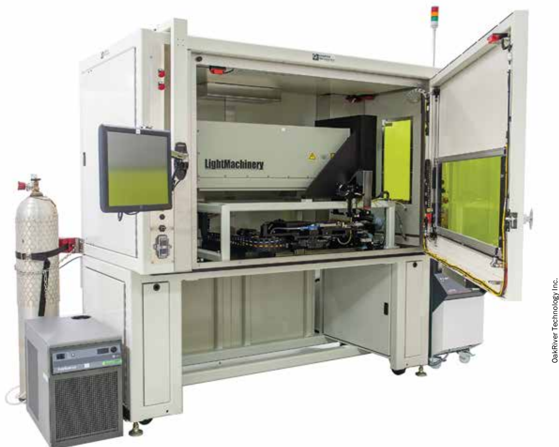
Figure 5. A typical integrated wire-stripping and cutting machine. Impact-2000 Series TEA CO 2 laser for stripping; Nd:YAG laser for cutting wire.
