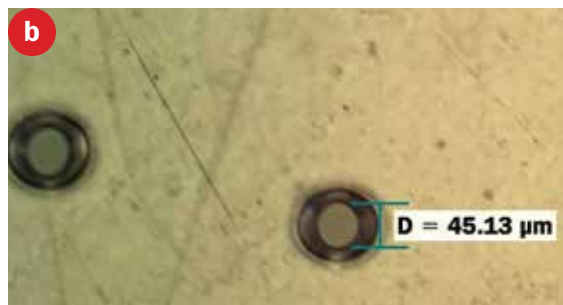
Figure 2. A comparison of excimer and TEA CO 2 processing of polyimide with 300-µm diameter holes (a) and approximately 50-µm holes (b). The use of a high quality compound lens was required to achieve these results. Some taper is to be expected in holes with a greater than 1:1 aspect ratio.
