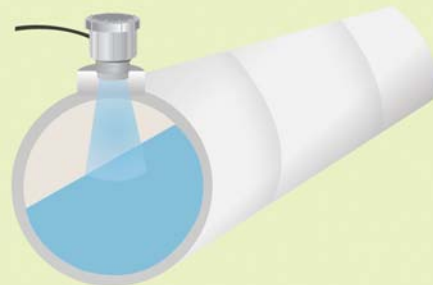
Water Level Measurement of Clean Water or Sewage
