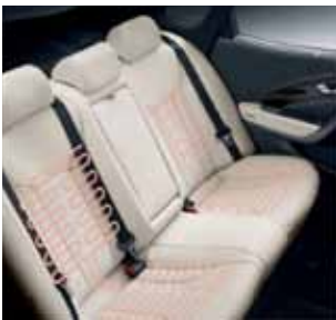
[Seat Heating Wire]
