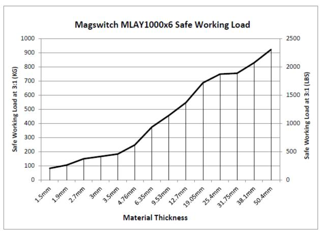
Note: Graph above shows performance of single tool. Heavy Lift Frame Series utilizes multiple magnets so consider number of tools when determining the capability of the tool.
