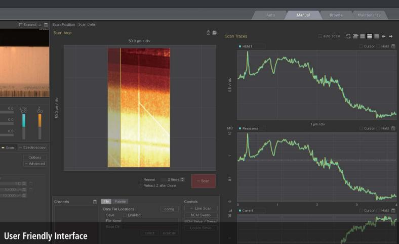
A large optical window provides easy to a view of the laser spot on the cantilever laser beam alignment on PSPD, and tip and sample positions. It also allow you to easily control the vision, the XY stage, Z stage, Optics stage, light strength and more on the CCD view.
