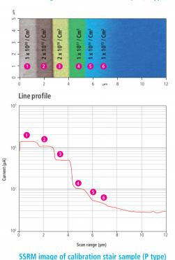
Park NX-Hivac allows failure analysis engineers to improve the sensitivity and resolution of their measurements through high vacuum SSRM. Because high vacuum scanning offers greater accuracy, better repeatability, and less tip and sample damage than ambient or dry N<sub>2</sub> conditions, users can measure a wide range of dope concentration and signal response in failure analysis applications.
