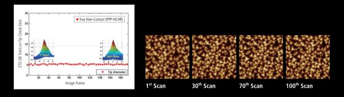
Furthermore, non-contact mode senses tip-to-sample force interactions occurring all around the tip. Forces occurring laterally to tip approach to the sample are detected. Therefore, tips used in non-contact mode can avoid crashing into tall structures that may suddenly appear on a sample surface. Contact and tapping modes only detect the force coming from below the tip and are vulnerable to such crashes.
