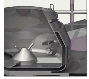
Agitator impeller lifting device
