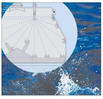
High pressure water is sprayed through purposefully placed nozzles to clean the inside of the vessel. The nozzles can be easily removed and reassembled.
