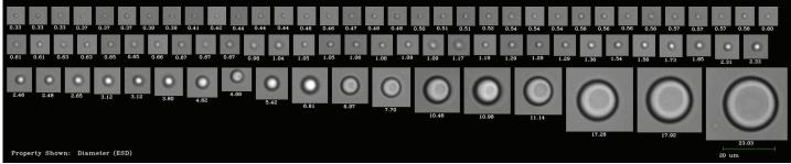
The above images are of a parenteral sample analyzed by the FlowCam Nano. The top image shows proteins 310 nm to 17.9  $\mu$ m in size and the bottom image shows silicon oil droplets 330 nm to 23  $\mu$ m in size. Diameter ( $\mu$ m) of each particle is noted beneath the each image. Particles can be sorted by 40+ parameters, including morphological charactersistics, using VisualSpreadsheet®.
