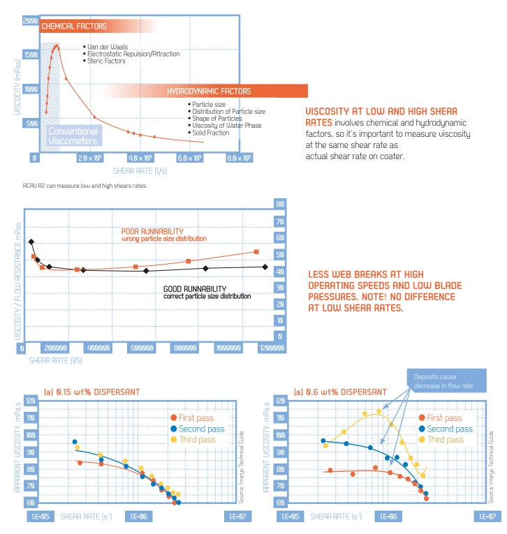
ACAV SLIT SHOWS EFFECT OF DISPERSANT DOSE ON SHEAR STABILITY OF COATING COLORS. KAOLIN + DISPERSANT, 10 PPH LATEX, 0.3 PPH CMC, 59 WT/ SOLIDS
