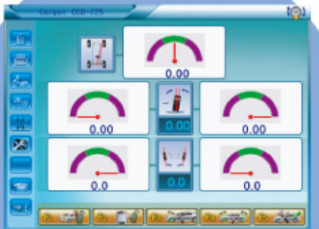
Adjusting Screen for Rear Adjustment screen including thrust angle
