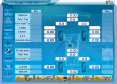
Measured Screen Helping decide how to adjust by showing whole condition with measured each values
