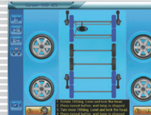
Runout procedure for different axes
