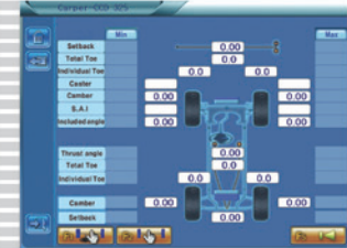
Measured data for different axes
