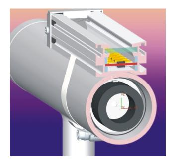
agnetic Type Level Indicator is an level. It has a magnetic float inside of the Non-Magnetic Chamber and an indicator outside of it.
