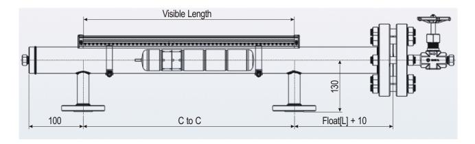
Float Lengths are totally difference depend on the specific gravity of liquid.
