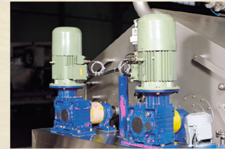
벡터방식 구동장치/VECTOR DRIVER DEVICE
