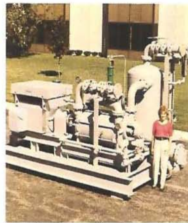
Large Condenser exhaustor system.
