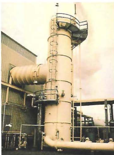
Direct contact geothermal condenser for 9 MW plant.
