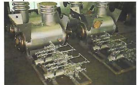
Condensers and air ejectors.
