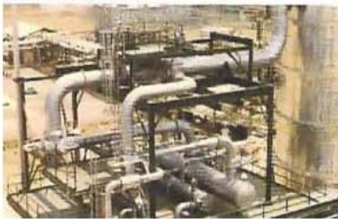
Ejectors in vacuum distillation service.
