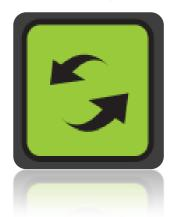
This key able to re-boot to all lamp's activation and deactivation. Press this key then press <u>SILENCE Key</u> again to maintain to each lamp's activation and deactivation. Or check buzzer sound activation
