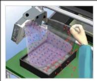
Removes Electrostatic charges generated When removing films
