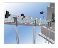
An Air-blow Ionizer Neutralizers Performs and Blows OFF Dust
