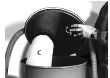
(A) Vacuum flow from receiver to blower; (B) Vacuum flow to receiver; (C) Filter
