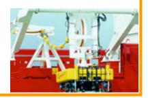
Umbilical floats are used in conjunction with ROVs to keep the required length of cable (dependent on the depth at which the ROV is operating) buoyant underwater.
