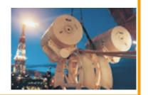
The Arch Structure is a steel framework within which sits a composite or steel buoyancy element. An arch can be used as a method to manage riser configuration.
