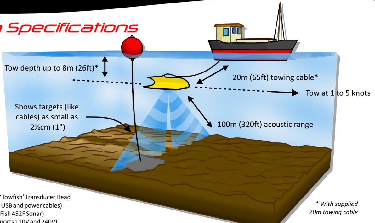
1. Starfish 452F Side Scan Sonar 'Towfish' Transducer Head
