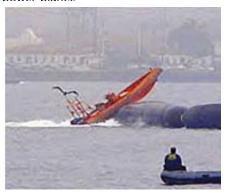
The unit once installed requires little maintenance and can be expected to have a life of 20 years or more. A barrier system currently in service was inspected on its 15th anniversary and certified as fully functional.
