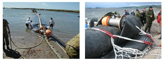
Initialy the Dracone Barge was used for military purposes involving the bulk water transportation of refined fuels. Commercial applications quickly followed and today, one of the most important functions of the Dracone is as an essential part of oil pollution control operations.
