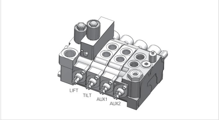
The main control valve for forklift truck is composed of several sections and valves. It controls fork lifting, master tilting, and auxiliary moving functions. The valve mainly functions as a directional control valve, but it also has several pressure and flow control valves, such as relief valve, flow regulator (down control) valve, tilt and lift lock valves. Also, additional safety functioning valves can be attached as in ISO type.
