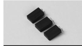
TCP is resistor that its resistance material is metal alloy wire wounded on ceramic core, then connected with Thermal fuse and this object with terminals inserted into the ceramic case which has good thermal conductivity.
