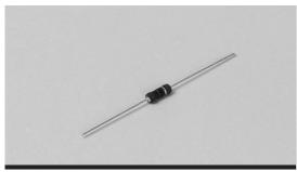
FNW is fusible wire wound resistor that is wound with special fusing wire on a high quality ceramic rod and protected by special high temperature silicon coating. This fusing type offering effect control surge is the most suitable for precision power circuit applications.
