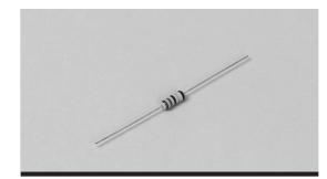
BCW is fusible wire wound resistor that is wound with special wire on a high quality ceramic rod and protected by special high temp Silicon coating. This resistor offering effect control In-Rush and Fusing, both are the most suitable for precision power circuit applications.
