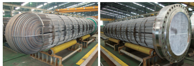
■ Tube Bundle of Heater
