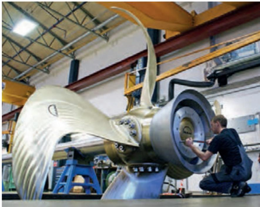
*MAN Alpha Kappel propeller – four-bladed CP with fairing cone for rudder bulb*
