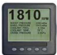
The ED-3 reads all engine data from the ECM and displays information in text and graphics. It includes full text alarm indication, data trending, internal buzzer and external alarm contact, as well as fault code logging with text description and service tool connection port.
