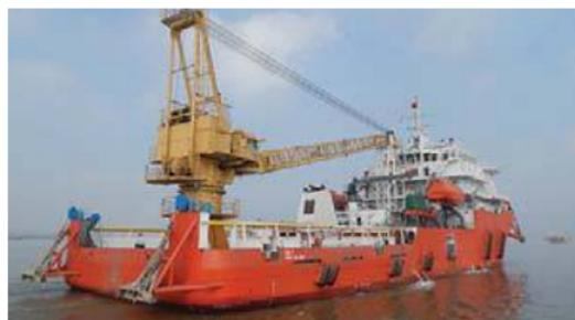
One of the two accommodation boats built at Guangzhou Mangtong Shipbuilding and outfitted with a pair of QSK60 main engines and three KTA38-powered generator sets.
