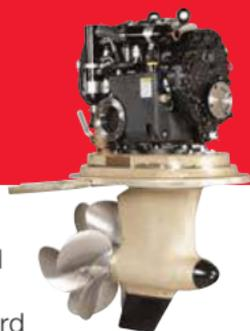
With SmartCraft innovation throughout, the Zeus<sup>®</sup> pod propulsion system provides a seamless approach to propulsion technology, marine electronics and on-board information management that makes boating safer and more enjoyable. Zeus offers dramatically improved high-speed handling and delivers up to:
