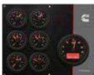
The gauge instrument panel provides fault code readout through a mini-digital display in the tachometer. This option displays coolant temperature, engine oil pressure, system voltage, exhaust stack temperature and gear oil pressure (if applicable). The GP is compatible with C Command Basic, Elite and Elite Plus\*
