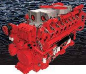
With ratings up to 4200 hp (3132 kW), Cummins QSK95 achieves power previously exclusive to medium-speed engines in a more compact installation. Innovative design makes it possible to provide 95 liters in a 78-liter platform weighing 25 to 70 percent less than medium speed platforms with similar power.
