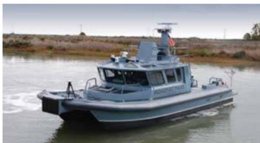
Also built by Moose Boats, this Bridgeport Police boat is powered by a pair of QSC8.3 main engines.
