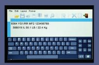
Hydra Software provides the easy to use WYSIWYG job display and the reliability of Windows XP. Patent pending Variable DPITM and nozzle flipping allows you to optimize the barcodes, text and logos optical density, speed and cartridge life. Add the optional ProPrint and now you have total control of your database as well. All the control you need at the printer or remotely.
