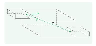
$$Attenuation = 10\log \left[ \frac{1}{Se(\cos\theta / 2\pi d^2) + (1-\alpha / \alpha S_w)} \right]$$
