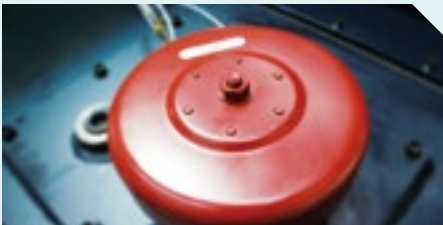
Air breather Easy access to air filter system on hydraulic tank.
