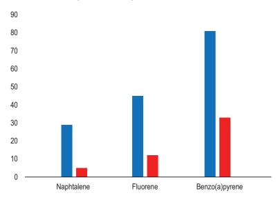
Relative immersion extraction yield (measured as % extracted after a 70 min) for PAHs at 50 ng/L with PDMS fibers (PAL SPME Arrow 100  $\mu$ m, 20 x 1.1 mm compared to SPME 100  $\mu$ m, 10 x 0.3 mm)
