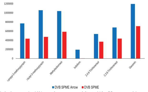
Relative headspace extraction yield (measured as amount extracted after 30 min) for off-flavor compounds in water at 100 ng/L with DVB fibers. (PAL SPME Arrow 100  $\mu$ m, 20 x 1.1 mm compared to SPME 100  $\mu$ m, 10 x 0.3 mm)
