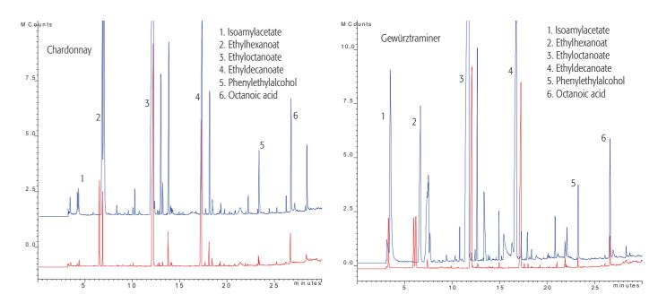
Chromatograms showing the headspace extraction of aroma components from different white wines with PDMS fibers (PAL SPME Arrow 100  $\mu$ m, 20 x 1.1 mm compared to SPME 100  $\mu$ m, 10 x 0.3 mm)
