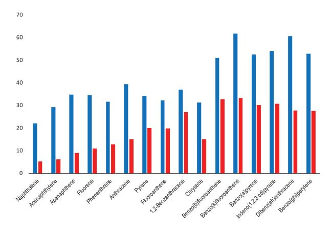
Extraction yields for water samples containing PAHs @ 50 ng/L after 70 min. A PAL SPME Arrow 20 mm x 250 µm Carbon WR was compared to SPME fiber 10 mm x 100 µm Carbon WR immersion (Kremser et al., 2015).
