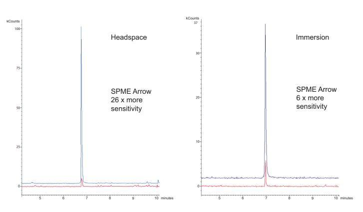
Extraction of 1  $\mu$ g/L iodoform from tap water with DVB fibers (headspace and immersion extraction), PAL SPME Arrow 100  $\mu$ m, 20 x 1.1 mm compared to SPME 100  $\mu$ m, 10 x 0.3 mm.
