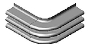
Round Corner - or best fatigue performance and best value. Rounded Corners U Profile Should be considered in applications up to 30 psig, and where vibration and cycle life are important factors. Rounded corners are the most expensive to manufacture. This design results in the lowest corner stress if fit up and welding of the corner seams are carefully controlled.
