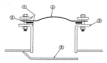
This type expansion joint is for flue gas which has passed through an air pre-heater and dust collector to reduce the temperature and particulate level. Flue gas may cycle near the dew point where condensation can occur and chemicals are present. Expansion joint may see thermal movement vibration and chemical attack.
