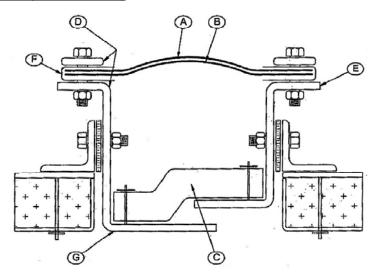
This type expansion joint is for flue gas directly after combustion stage at elevated temperatures with possible particulate present. Expansion joint is used for possible large thermal movements at elevated temperatures.
