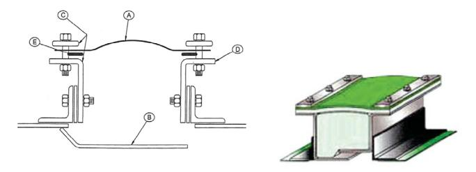
Ambient temperature clean air without particulate or chemicals to damage the flexible element. Expansion Joint is used frequently for vibration and sound attenuation from fan equipment.
