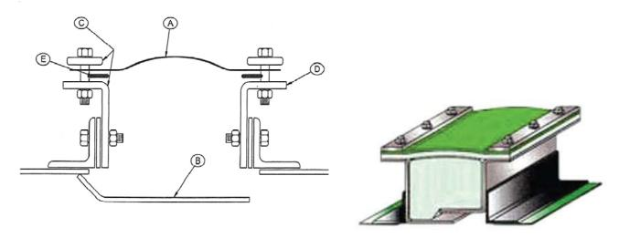
Clean air, after coming into contact with hot flue gases at the air pre-heater where temperatures are elevated with minimal particulate and or gas carryover. Expansion joint will see thermal movements and vibration. Elevated temperatures require a composite flexible element and a flow liner.
