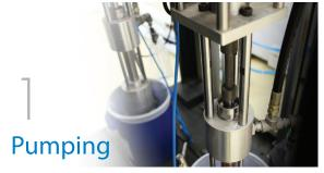
Deliver raw material divided into A part and B part to mixing block through exclusive pipe on dosing pump
