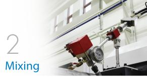
Mix gathered main material and hardener through static mixer, then provide material to Cool runner with pressure limiter adjusting dosing time and material amount regularly
