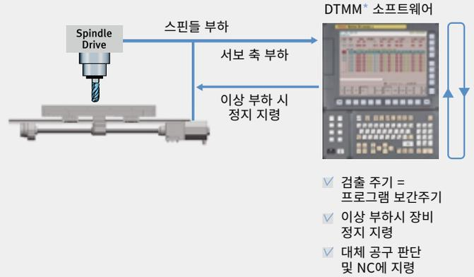
\*DTMM : DN Solutions Tool load Monitoring for Machining Centers
